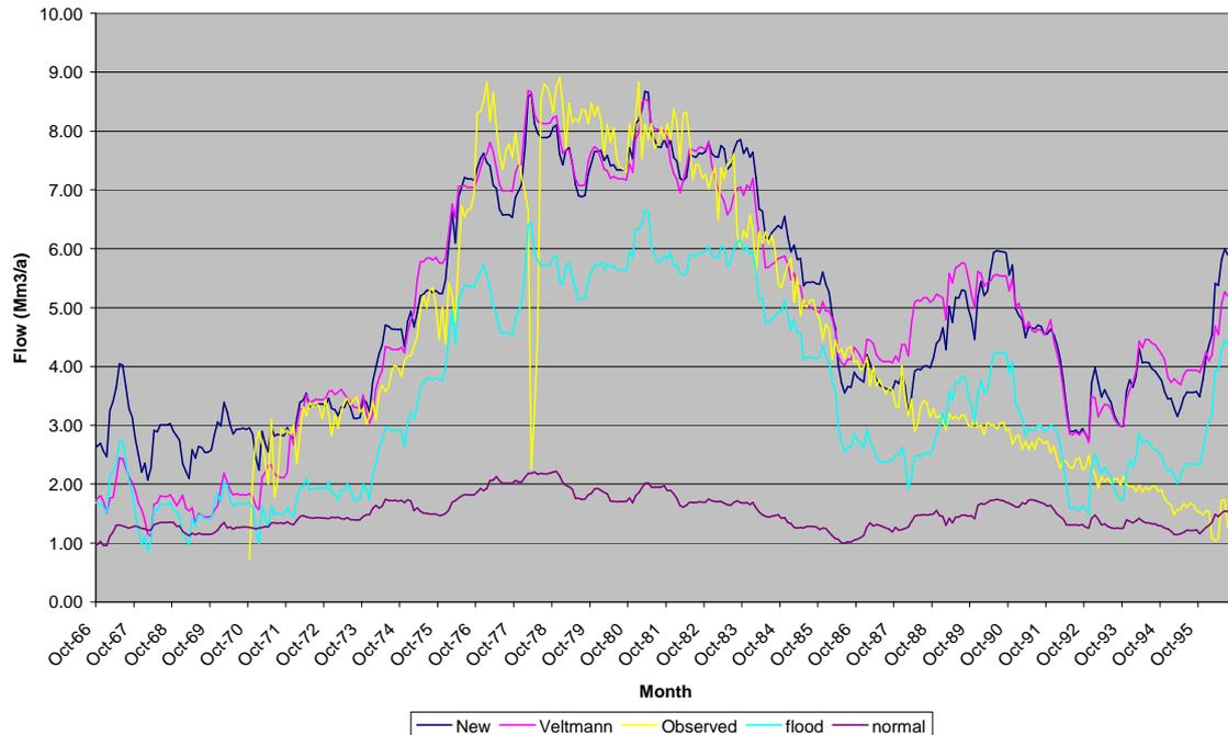
Figure1: Calculated spring discharge used in this study (new) compared to the Veltman study, as well as flood (ReF) and normal recharge (ReN).
