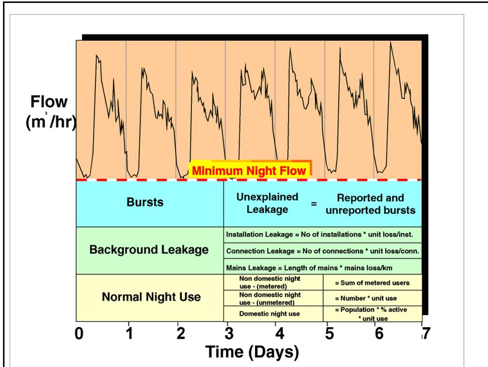
Figure 4: Components making up the minimum night-flow
