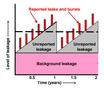
Figure 2: Simplified BABE components of SRELL, varying with time, assuming regular survey
