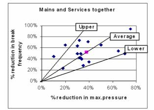
Figure 4: Simple basis for predicting % reduction in breaks from % reduction in maximum pressure
