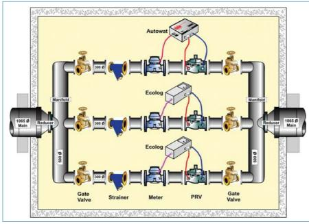
Figure 2. Schematic Layout of the 1065 mm diameter Installation.
