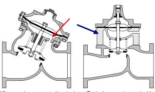
"Y" type valve, converted to single chamber design by opening bores in the bottom chamber
