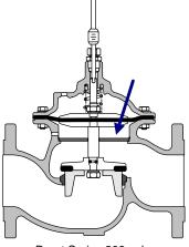
Dorot Series 300 valve, converted to DC design by adding aseparation disc
