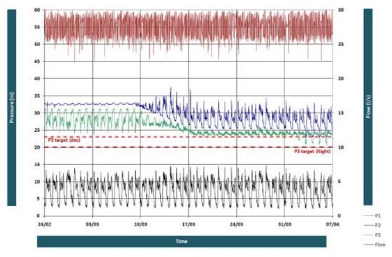
Figure 1.4: Pressure and flow in Coviolo dma
