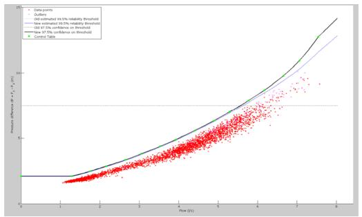
Figure 1.5: Recorded flow related pressure between the PRV outlet and critical point in Coviolo dma
